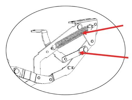
Leg extending spring strengthens the supporting force of footrest when the leg is stretched out and ensures better self-locking performance when the leg is retracted.
